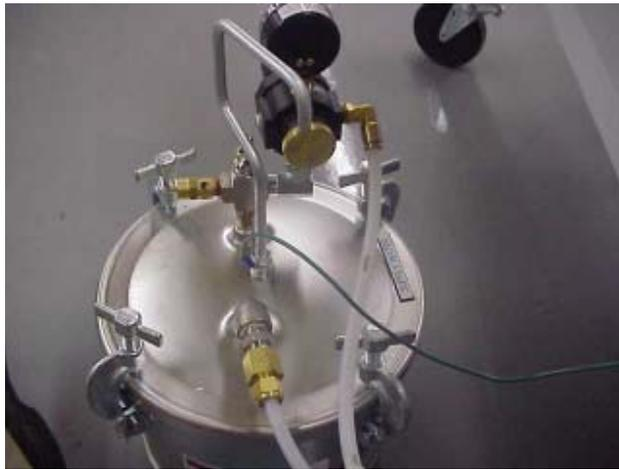
**Figure 3: Fluid and Air Line Connections**
